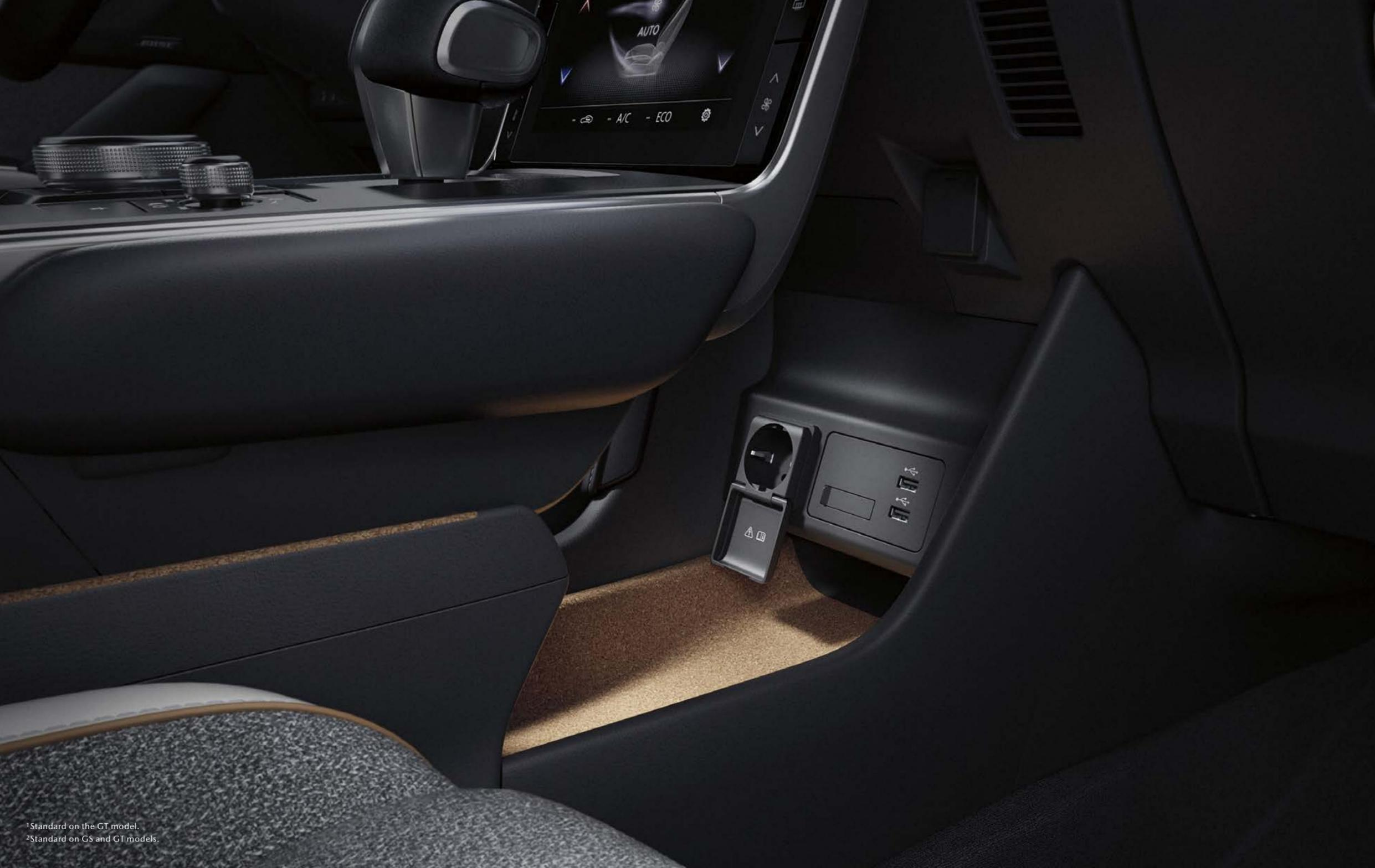
**Left:** 120 V 150 W AC power outlet<sup>1</sup> and dual USB ports,<sup>2</sup> under the floating centre console
